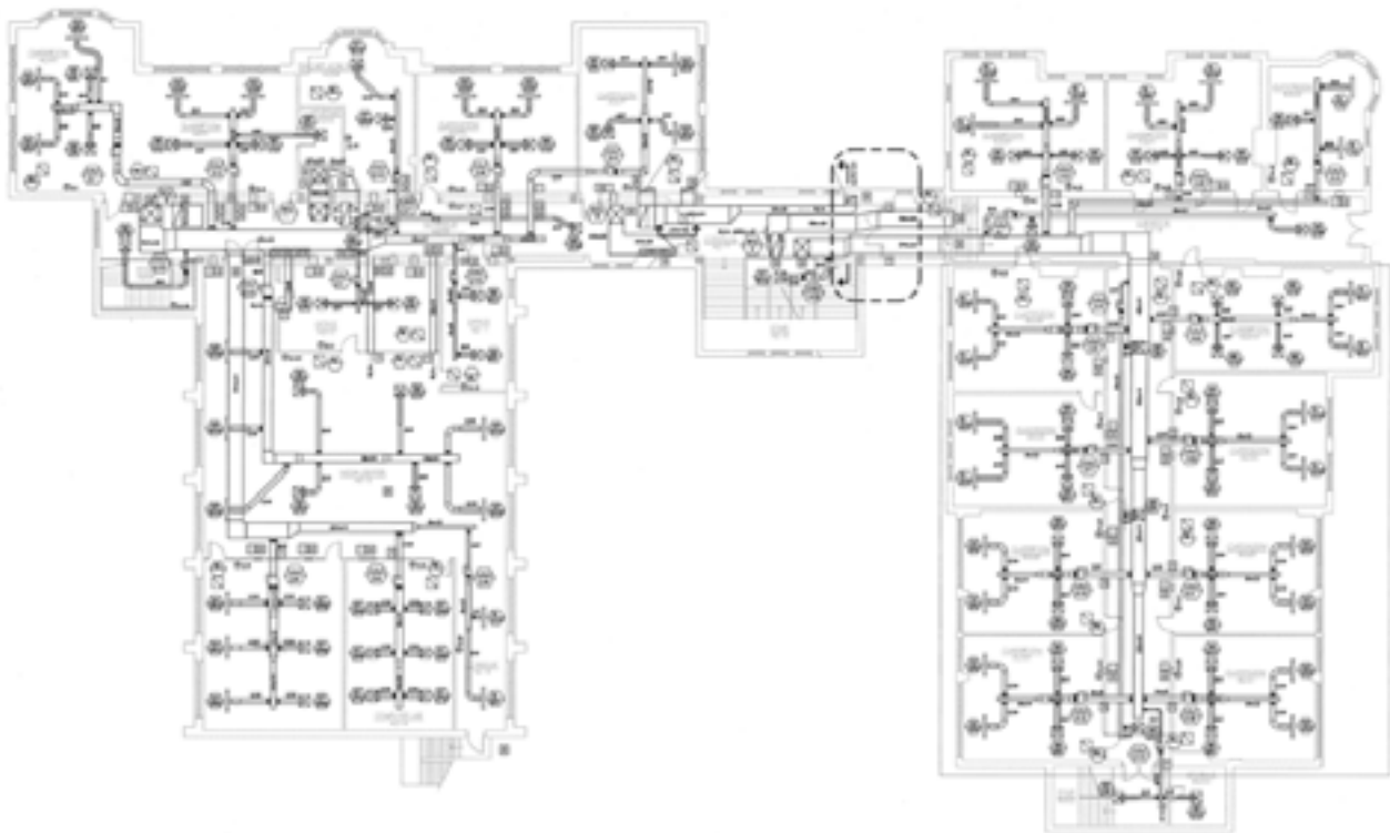
Harrisburg High School VAV System
