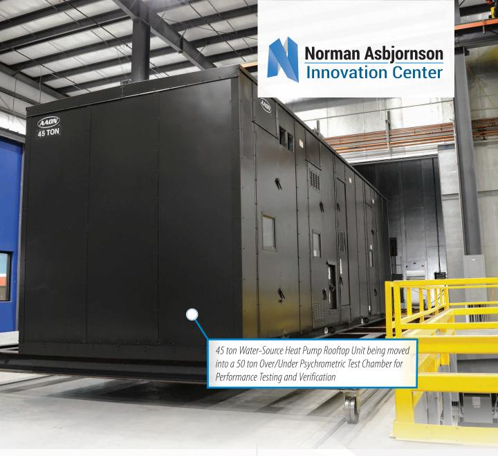
Verified performance provides assurance that your building's HVAC equipment will perform as specified. The Norman Asbjornson Innovation Center is the only lab in the world capable of testing thermal and acoustic performance under actual load conditions, for HVAC equipment up to 540 tons.
