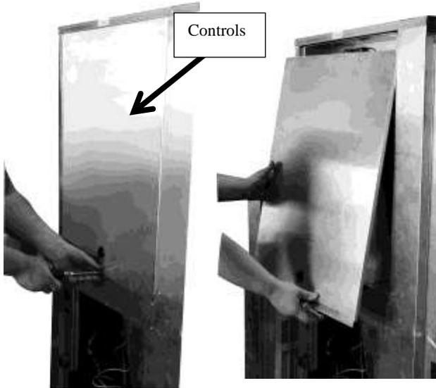
2) Using a  $\frac{5}{16}$ " socket, remove the screws on the outside of the control panel.
