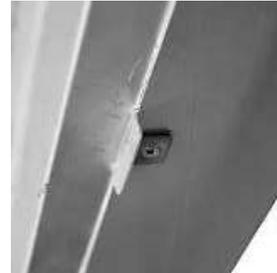
Figure 9 - Pre-cut Aluminum Handles bent to 90 degrees
